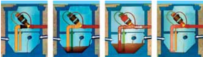
Above: valve operation scheme.
