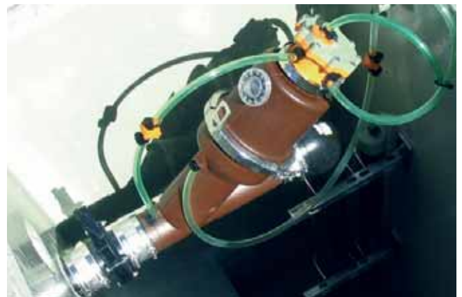
In the photo: particular of the automatic interface valve.
